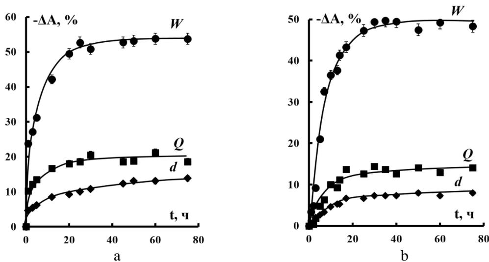
Figure 1. The kinetic dependences of the relative changes in moisture content ( $W$ ), total exchange capacity ( $Q$ ) and thickness ( $d$ ) of the membranes  $MK-40_{pr}$  (a) and  $MA-40_{pr}$  (b) after contact with the phenylalanine solution of concentration  $C_0=0.15\text{mol/dm}^3$ .
