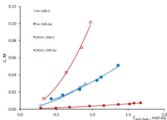
Figure 3. Depending concentration of sodium ions in solutions of acid and sulfate ions in solutions of alkali on concentration of solutions of acid or alkali, produced in EDA containing bipolar membranes MB-3 or MB-2m and monopolar membranes Ralex CMX and Ralex AMH.
