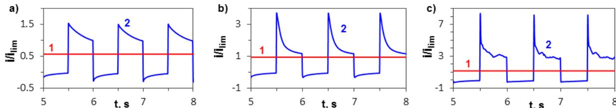
Figure 3. Dependences of the current density on time at the quasi-stationary (1) and PEF (2) regimes for the average potential drop equals  $U_{av} = 0.1$  V (a),  $0.45 \text{ V}$  (b),  $0.65 \text{ V}$  (c).
