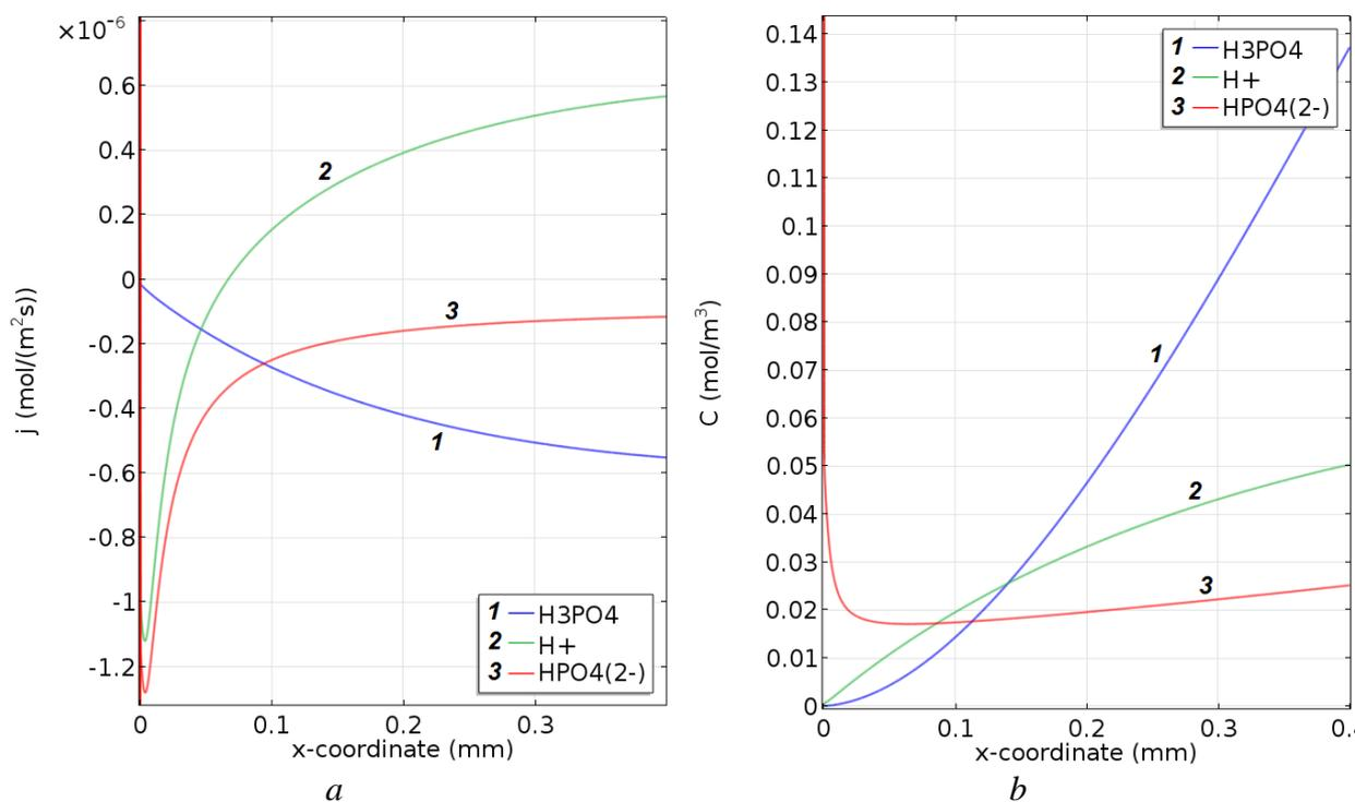
Figure 2. Fluxes (a) and concentrations (b) of  $\text{H}_3\text{PO}_4$ ,  $\text{H}^+$  and  $\text{HPO}_4^{2-}$  for  $\text{NaH}_2\text{PO}_4$  solution with concentration  $20 \text{ mol}/\text{m}^3$  at a given potential drop in the diffusion layer  $d_\phi = -0.2\text{V}$ .
