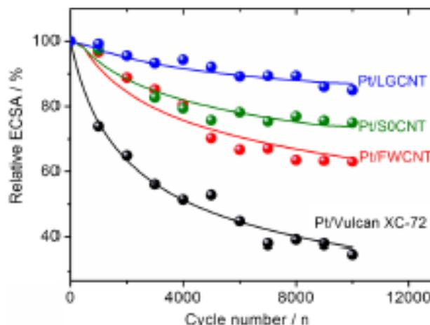
Figure 2. Relationship between the ECSA and the cycle number during the APCT.
