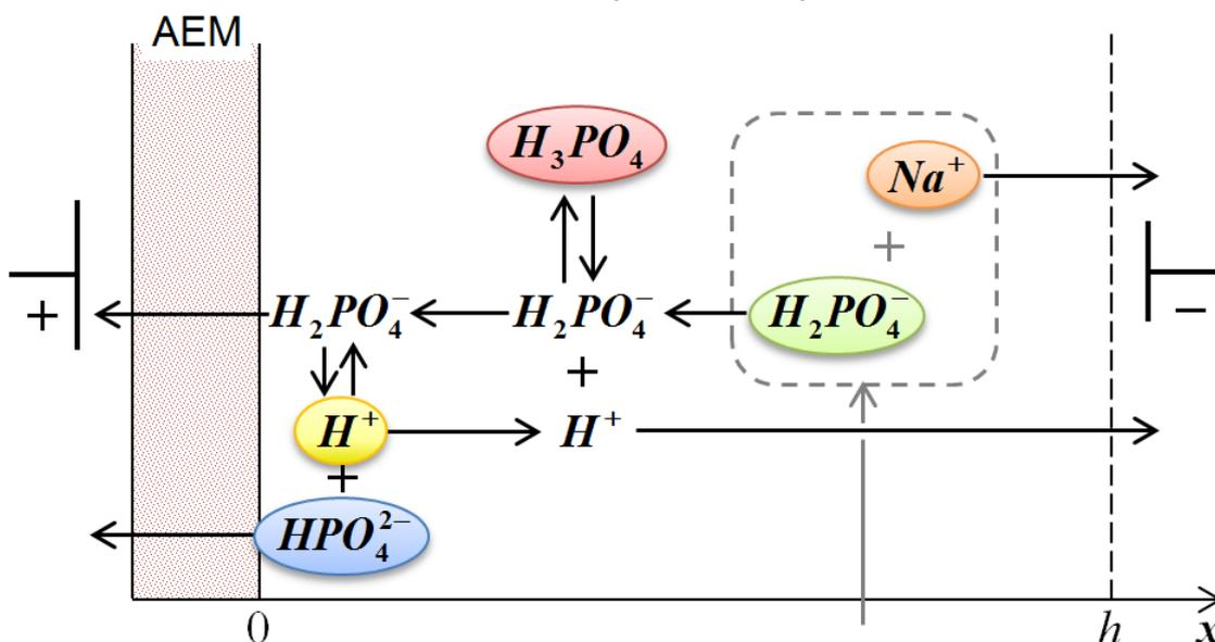
Figure 1. Scheme of the ions transport in the diffusion layer.
