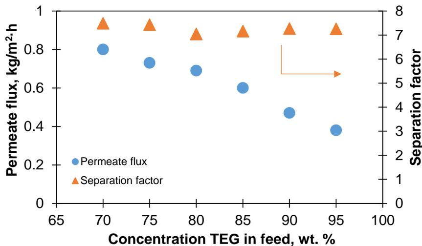
Figure 2. Dependences of permeate flux and separation factor on concentration TEG in feed,  $T_f = 60\text{ }^\circ\text{C}$ ,  $T_c = 10\text{ }^\circ\text{C}$ ,  $l_{air\ gap} = 2.0\text{ mm}$ .
