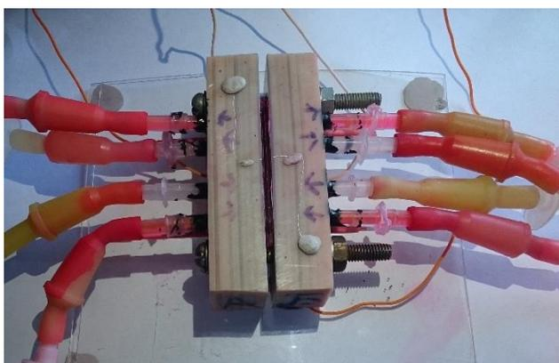
*Figure 1. Image of the Electrodialysis Cell Developed for Visualization of Electroconvective Vortex.*
