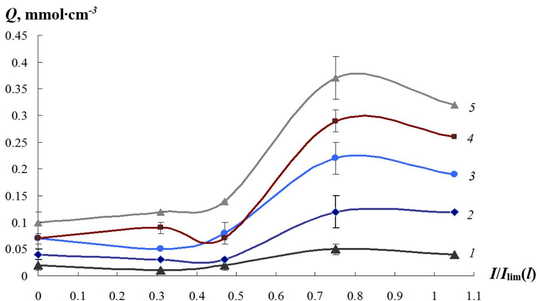
Figure 2. Reduction oxygen quantity on  $Cu^0$ -Lewatit K2620( $Na^+$ ) nanocomposite at the time  $t$ ,  $h$ : 1 – 1; 2 – 2; 3 – 3; 4 – 4; 5 – 5. Experiment conditions:  $l = 1 \cdot 10^{-2} m$ ,  $u = 0.23 cm/sec$ ,  $I_{lim}(l) = 2.9 mA$ . Experiment time is 5 h.
