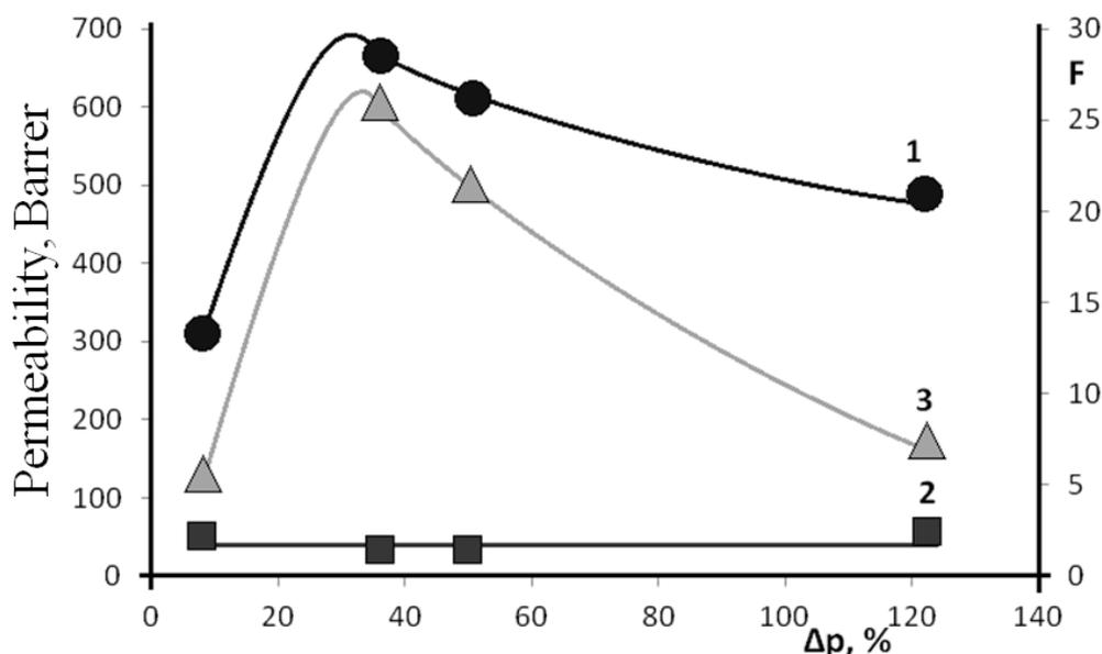
Figure 1. The permeability coefficients dependence of gases recovered from the isobutylene and butane mixtures of composition  $C_4H_8/C_4H_{10} = 10:90$  v/v. on the membrane PS grafting degree: 1 - isobutylene permeability, 2 - butane permeability, 3 - isobutylene - butane mixture separation factor. Relative humidity - 80%.
