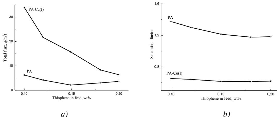
*Figure 4. Dependence of (a) total flux and (b) separation factor(thiophene/heptane) on thiophene concentration in the feed for pervaporation of n-heptane-thiophene mixture using membranes: PA and PA-Cu(I), 20 °C.*
