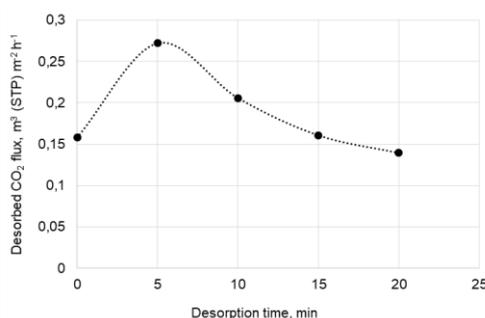
Figure 2. The flux of CO<sub>2</sub> desorbed in porous membrane contactor vs. time of desorption experiment.
