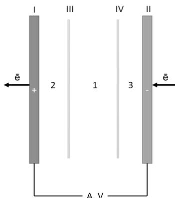
Figure 1. Scheme of RED lab-scale. I – anode, II – cathode, III – anion-exchange membrane, IV – cation-exchange membrane, A – ammeter, V – voltmeter, 1 – dilution chamber, 2 – pre-anode chamber, 3 – pre-cathode chamber.
