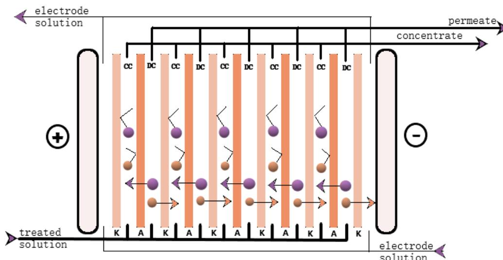
Figure 1. Diagram of the process of electro dialysis.
