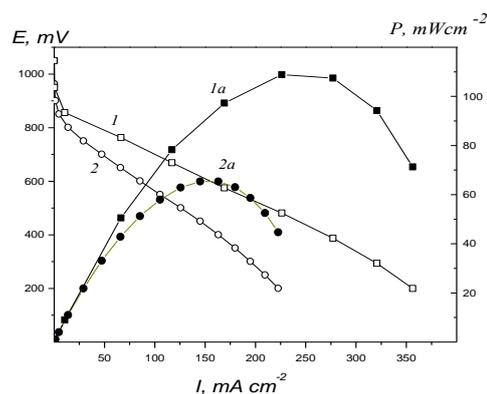
Figure 4. The current-voltage (1, 2) and power (1a, 2a) characteristics of the FC based on the UHMWPE-sPS (1, 1a) and Nafion-115 (2, 2a) membranes.
