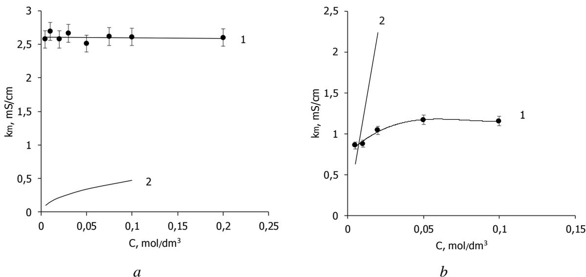
Figure 2. Concentration dependence of the electrical conductivity of ion-exchange membranes in solutions of acetic acid (a) and sodium chloride (b): 1 - MA-41; 2 - electrolyte solution.
