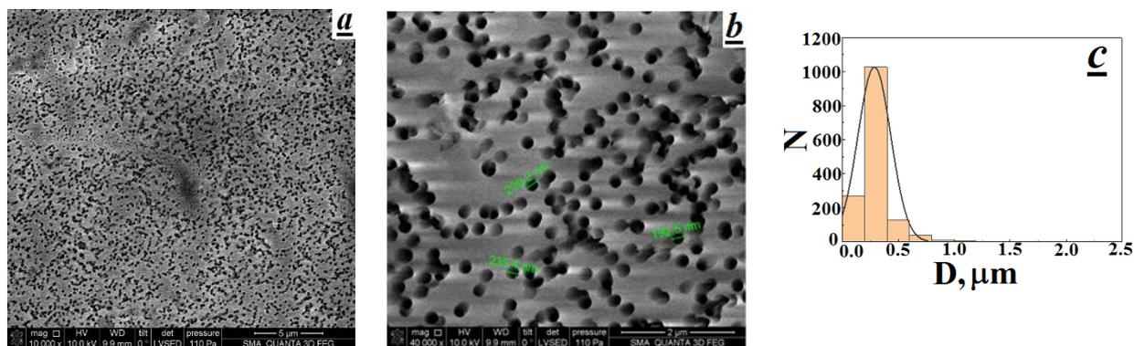
Figure 1. a, b) Electron microscopic images of the nuclear filter samples surface irradiated by xenon ions with an energy of  $\sim 1 \text{ MeV/nucleon}$  to  $\sim 3 \times 10^8 \text{ cm}^{-2}$  polyethylene terephthalate films, after chemical treatment in aqueous solutions of 5N NaOH at 343 K for three minutes; c) pore size distribution function and the result of its approximation by a lognormal distribution.
