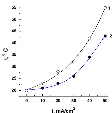
Figure 2. The dependence of the increment of temperature on time at a current density of at electro dialysis 0.05 M solution of potassium chloride (solid circles show the increment of temperature in the sections of desalination and hollow circles sections concentrating).
