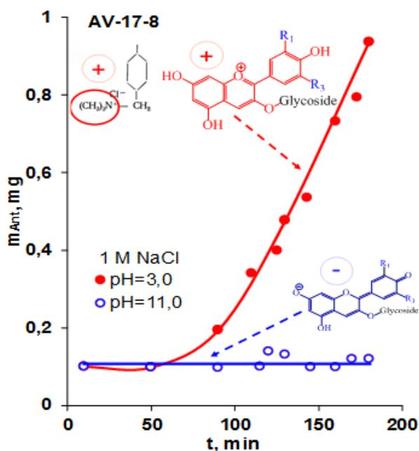
Figure 2. The Kinetics of Anthocyanins Desorption from AV-17-8 Using 1M NaCl Aqueous Solution with pH value 3,0 and 11,0.
