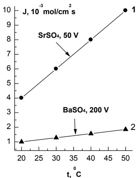
Figure. 1. The dependence of the fluxes of ions of strontium (1) and barium (2) in electro dialysis of sulphate suspensions on the temperature at a voltage of 50 (1) and 200 (2) with alternating anion exchange and cation exchange membranes MA-40 and MK-40.
