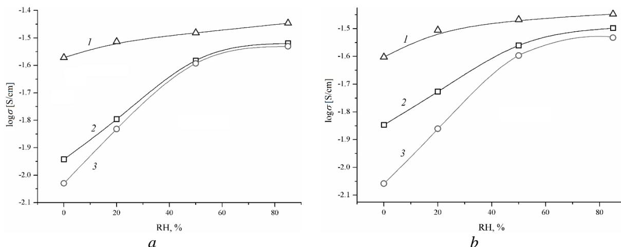
Figure 1. Plots of conductivity versus relative humidity at 90°C for the PBI-O-PhT (1), PBI-2,5Py (2), PBI-2,6Py (3) membranes containing 15 wt% of SiO<sub>2</sub>Im-ex (a) and 15 wt% of SiO<sub>2</sub>Im-in (b).
