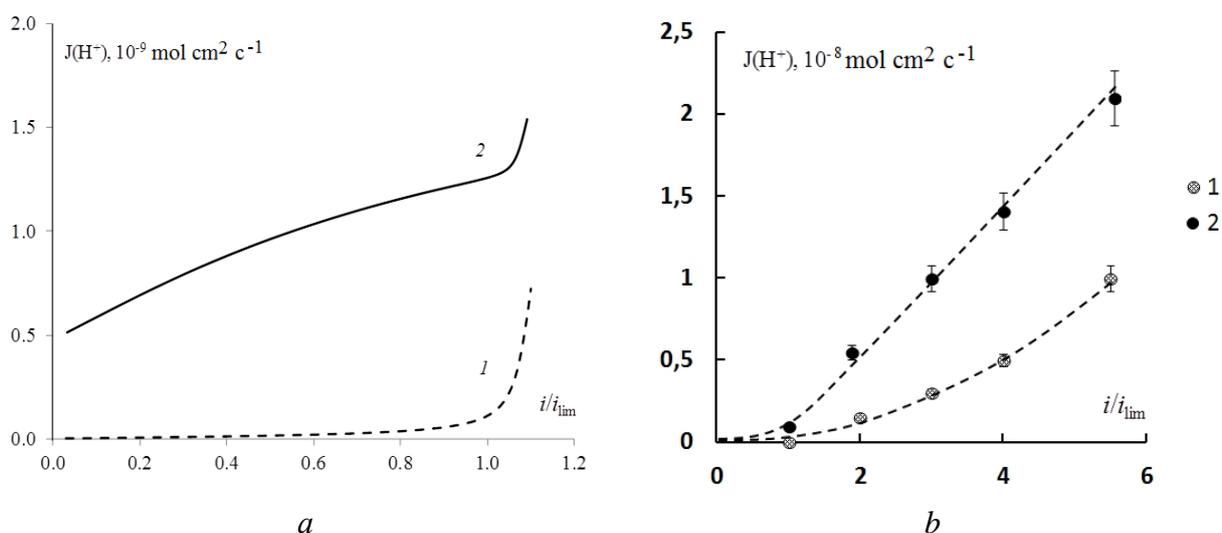
Figure 2. Hydrogen ions flux through the cation-exchange membrane vs. dimensionless current density curves: a - numerical simulation results (1 - salt is not subjected to hydrolysis in aqueous solution; 2 - salt is formed by a weak base); b – experimental results (1 -  $\text{KNO}_3$ , 2 -  $\text{NH}_4\text{NO}_3$ ).
