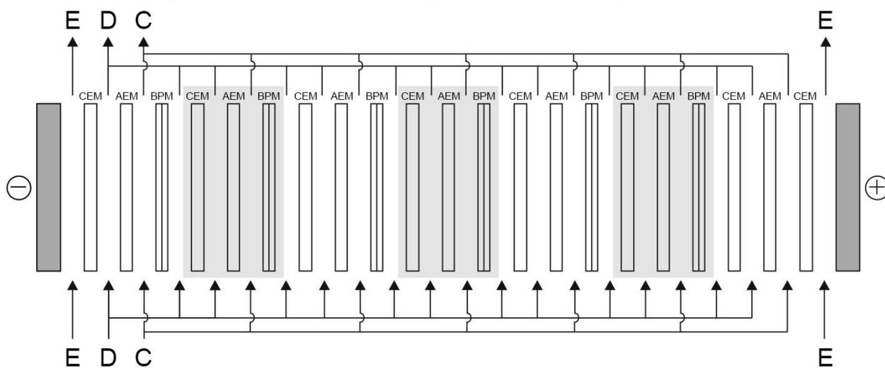
Figure 1. ED cell for acid whey treatment. E, D and C indicate electrode solution, diluate and concentrate stream, respectively; CEM, AEM and BPM are cation-exchange, anion-exchange and bipolar membranes, respectively.
