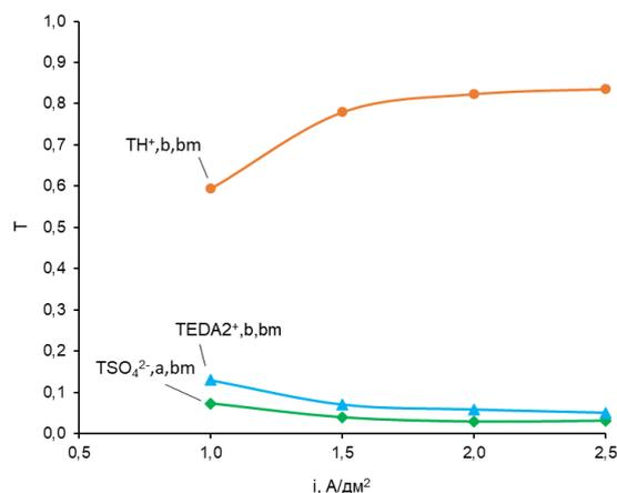
Figure 6. The dependence of the effective transport numbers of ion through the bipolar membrane on the electric current density in the system " ethylenediamine, ethylenediamine sulfate – H<sub>2</sub>SO<sub>4</sub>».
