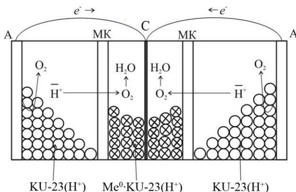
Figure 2. The scheme of processes in deoxygenator (sorption-membrane electrolyzer with the granular layer of NC): A – anode, C – cathode, MK – sulfocation-exchange membrane.
