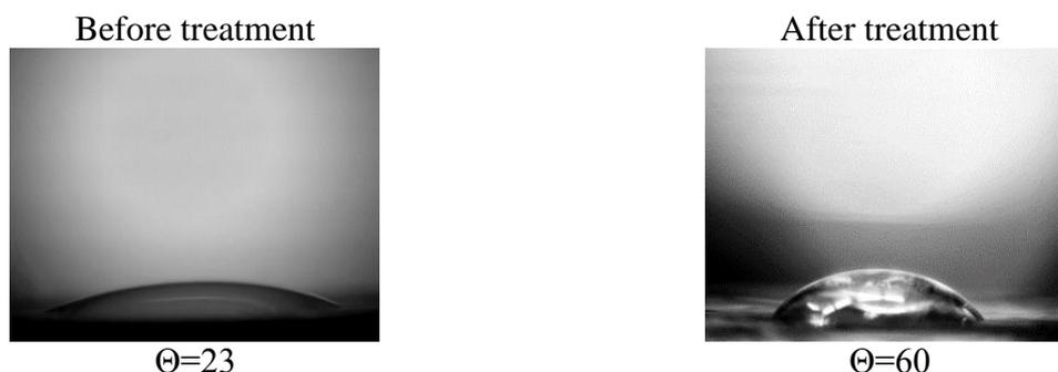
Figure 2. Images of tetraethylene glycol dimethyl ether droplets on the surface of cellophane before and after Protect Guard treatment.
