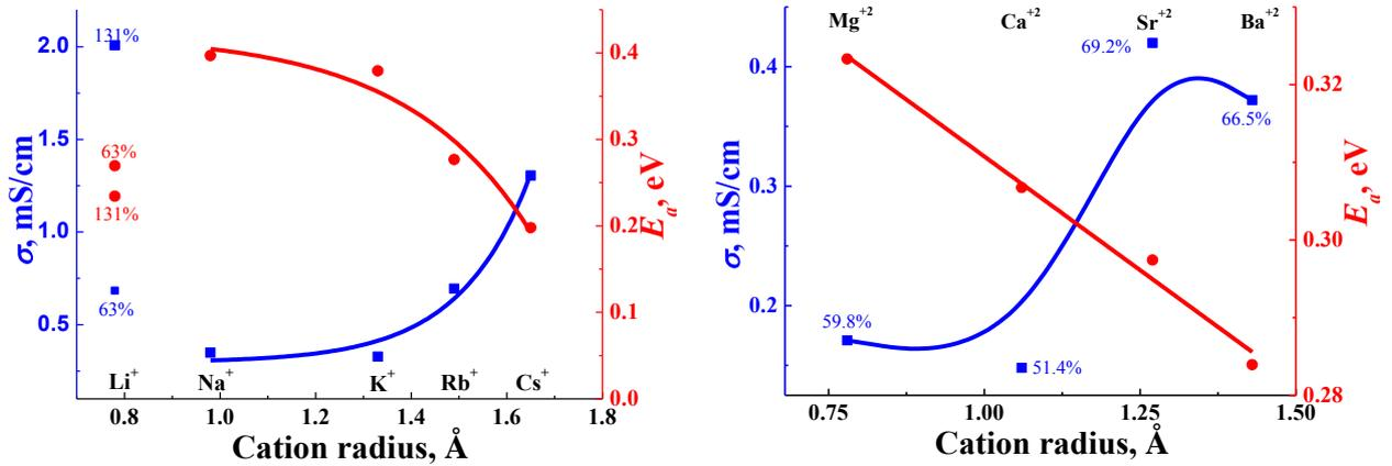
Figure 1. Dependence of conductivity and activation energy of conductivity of Nafion-M<sup>Z+</sup> membranes plasticized by DMSO on cation radius. Percent show the swelling degree.
