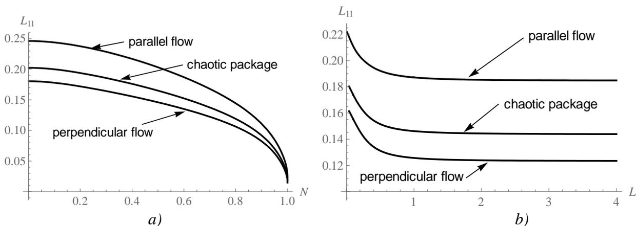
Figure 2. Variation of the dimensionless hydrodynamic permeability  $L_{11}$  of a membrane with the parameters  $N$  (a) and  $L$  (b) for  $\sigma = 3$ ;  $\varepsilon = 0.75$ ;  $a / b = 0.5$ ;  $c / b = 1.5$ .
