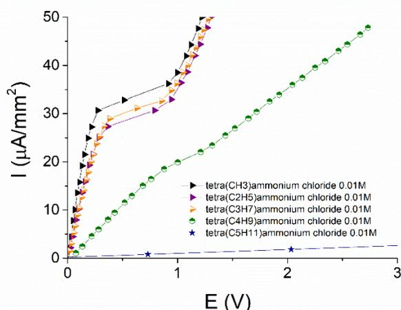
Figure 1. DOWEX™ HCR-S/S current-voltage curves for aqueous solutions of tetraalkylammonium chlorides of increasing size.
