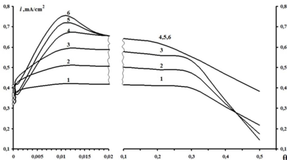
Figure 2. Dependence of the current density in terms of salt ions on the fraction of inert regions on the membrane surface for different values of electric potential jump  $\Delta\phi$ : (1) 0.4, (2) 0.5, (3) 0.6, (4) 0.7, (5) 0.8, and (6) 0.9 V.
