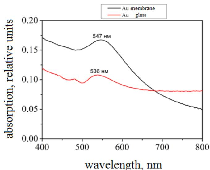
Figure 3. Au nanoparticle absorption spectra.
