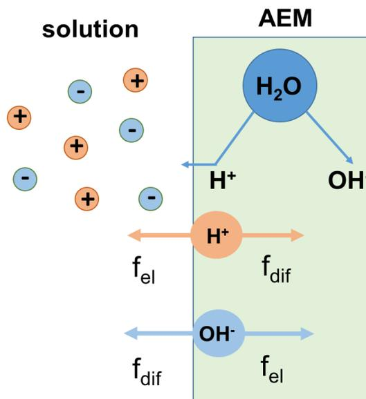
Figure 2. Scheme of pH Shift in an Anion-Exchange Membrane.
