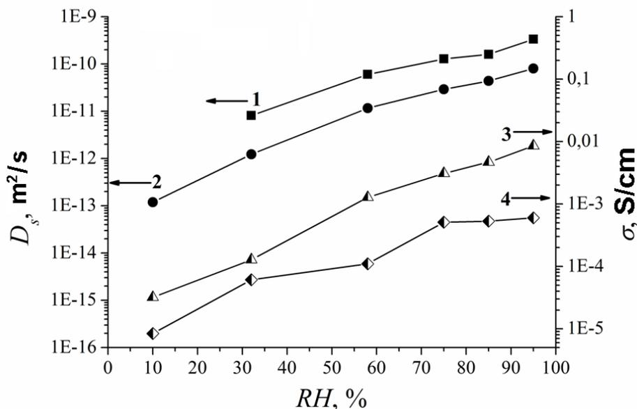
Figure 1. Humidity dependence of water molecule self-diffusion coefficients (curve 1);  $\text{Li}^+$  self-diffusion coefficients (curve 2); ionic conductivity calculated from Nernst-Einstein equation (curve 3) and experimentally measured (curve 4) in  $\text{Li}^+$  form of Nafion.
