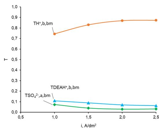
Figure 5. The dependence of the effective transport numbers of ion through the bipolar membrane depending on the electric current density in the system " diethylamine, diethylamine sulfate–H<sub>2</sub>SO<sub>4</sub>».
