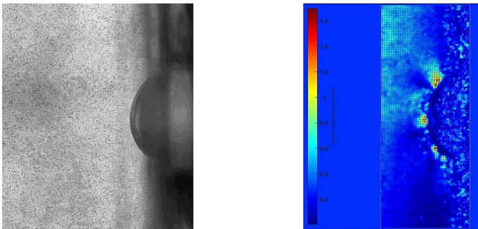
Figure 4. Electroconvection velocity magnitude map for DOWEX™ HCR-S/S particle in the solution of tetrapentylammonium chloride 0,01M during the CVC measurement.
