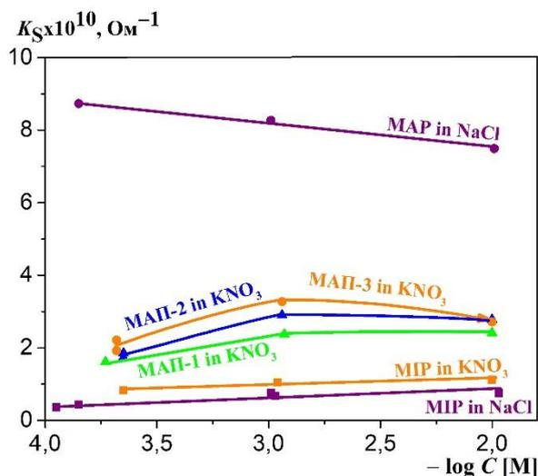
Figure 1. Dependencies of specific surface conductivity of iron-containing Fe-4 porous glasses on the concentration of NaCl[1] and KNO<sub>3</sub> solutions.
