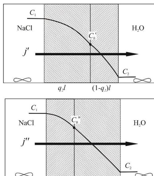
Figure 2. Schematic presentation of the system “bi-layer membrane – NaCl” solution with considering the different orientation of the membrane towards the electrolyte flux.
