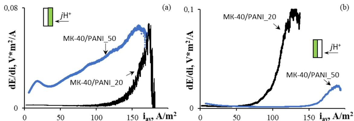
Figure 2. Derivative of I-V curve,  $dE/di$  vs  $i_{av}$ , for membranes synthesized at  $i=20$  (MK-40/PANI\_20) and 50 (MK-40/PANI\_50)  $\text{mA/cm}^2$ : modified (a) and non-modified (b) surface layers are placed towards desalination chamber.
