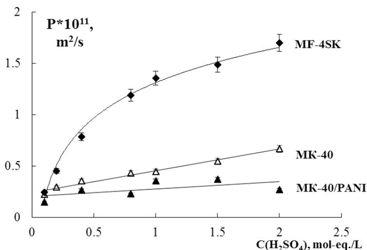
Figure 1. Concentration dependences of diffusion permeability of the MK-40, MF-4SK and MK-40/PANI membranes in sulfuric acid solutions.
