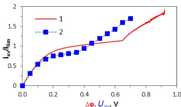
Figure 2. CVC (1) and dependence of the average current density on potential of the PEF (2).
