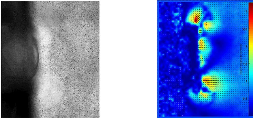
Figure 3. Electroconvection velocity magnitude map for DOWEX™ HCR-S/S particle in the solution of tetramethylammonium chloride 0,01M during the CVC measurement.
