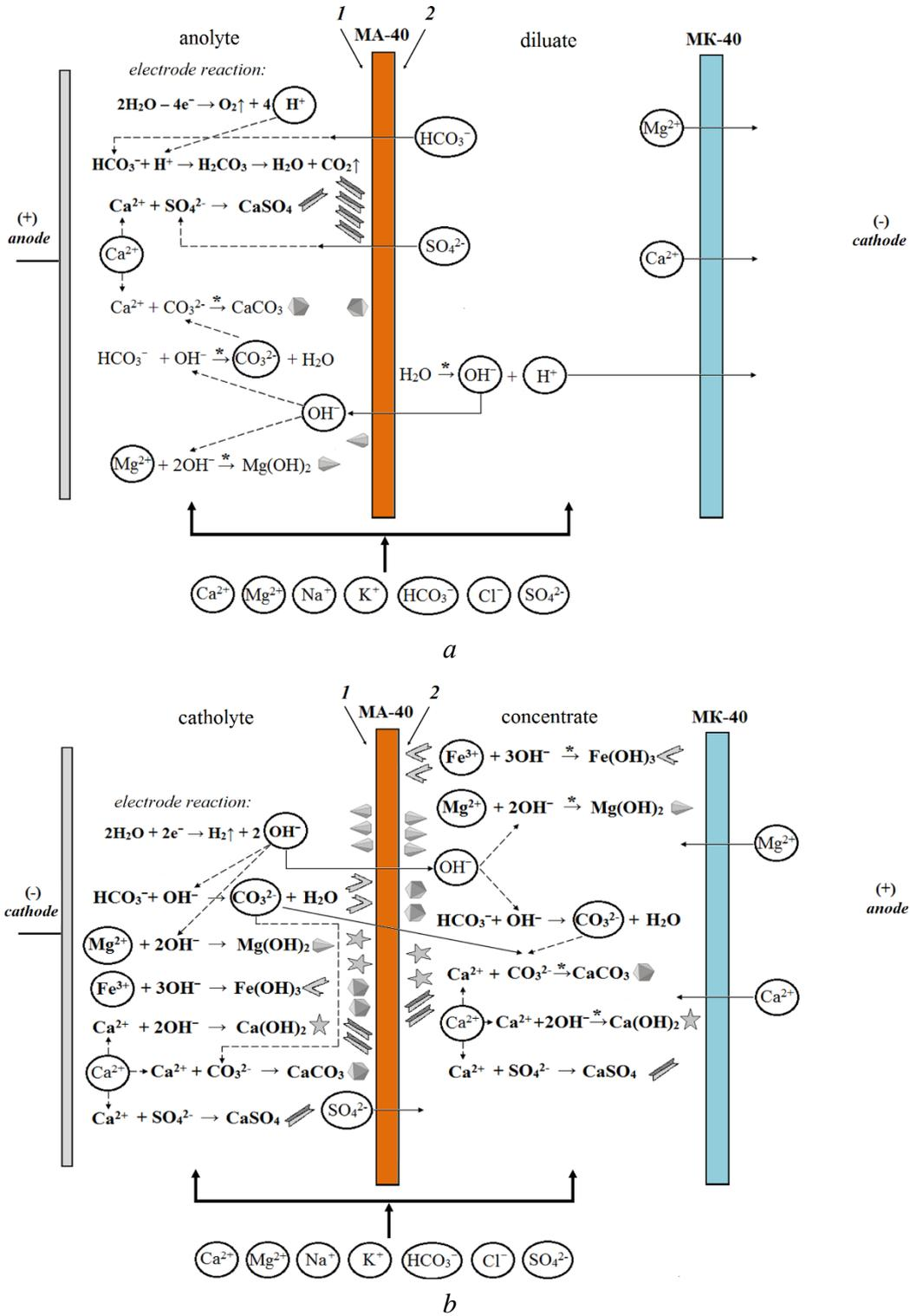
Figure 2. The general scheme of the precipitate formation during operation of the electro dialyzer in the modes of direct (a) and reverse (b) current. \* - reactions occurring at the solution – membrane interface. The numbers 1 and 2 show the designation of the membrane sides.
