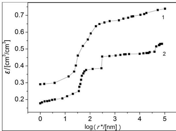
Figure 1 Integral pore size distributions for the electrode based on Norit carbon. The curves are plotted as pore volume vs effective pore radius. Working liquids: octane (1) and water (2).
