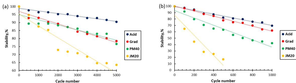
Figure 1. Stability change during voltammetry stress-test in potential range (a) 0.6 – 1.0V (b) 0.6 – 1.4V. 0.1 M HClO<sub>4</sub>, Ar atmosphere.
