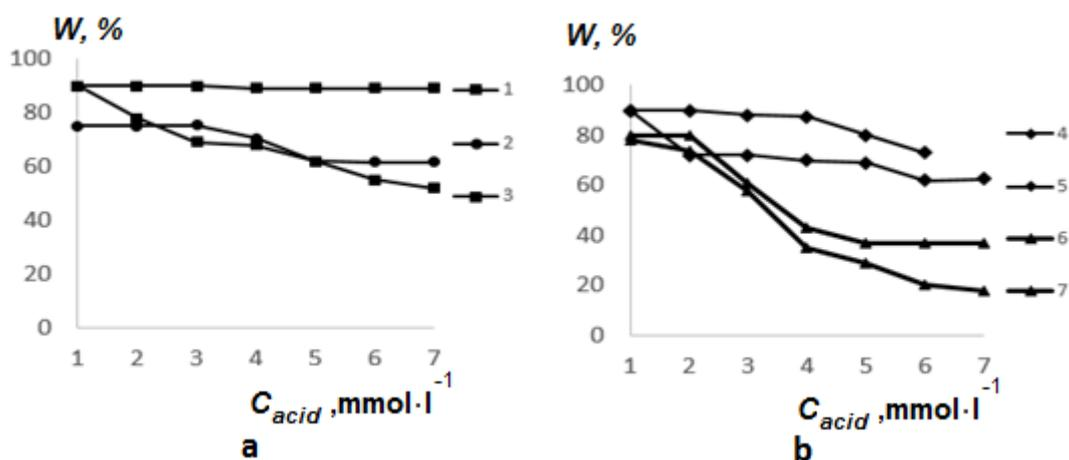
Figure 1. Influence of the nature and concentration of acids on the degree of extraction of Au (III) ions in  $\text{H}_2\text{SO}_4$  (1) and  $\text{HCl}$  (3), Ag (I) in  $\text{HNO}_3$  (2), Pd (II) in  $\text{H}_2\text{SO}_4$  (4) and  $\text{HCl}$  (5), Pt (IV) in  $\text{H}_2\text{SO}_4$  (6) and  $\text{HCl}$  (7).
