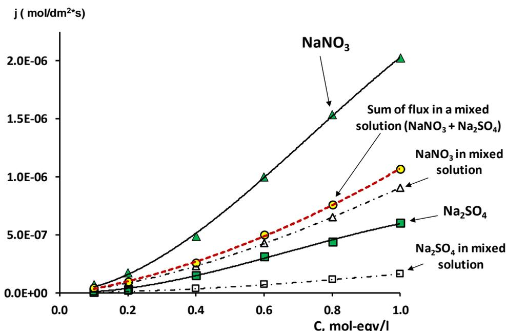
Figure 2. Dependence of the diffusion flow of salt through the membrane of MF-4SK on the concentration of salt.
