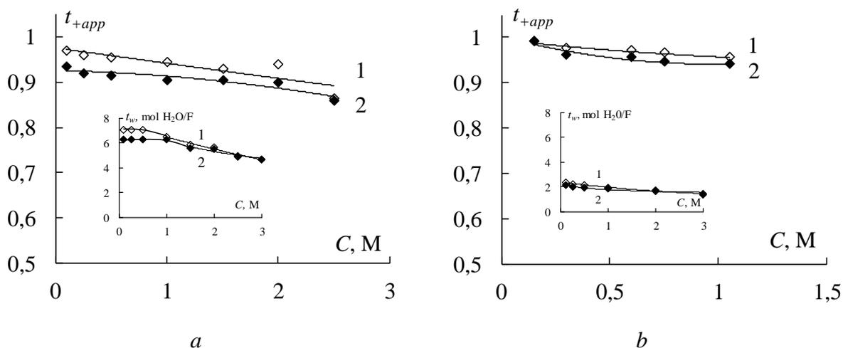
Figure 1. Concentration dependences of apparent transport numbers counterions and water transport numbers for MK-40 (1) and MK-40/PANI (2) membranes in NaCl (a) and HCl (b) solutions.
