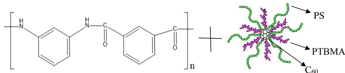
Figure 1. Structures of PA and hybrid star-shaped macromolecule.
