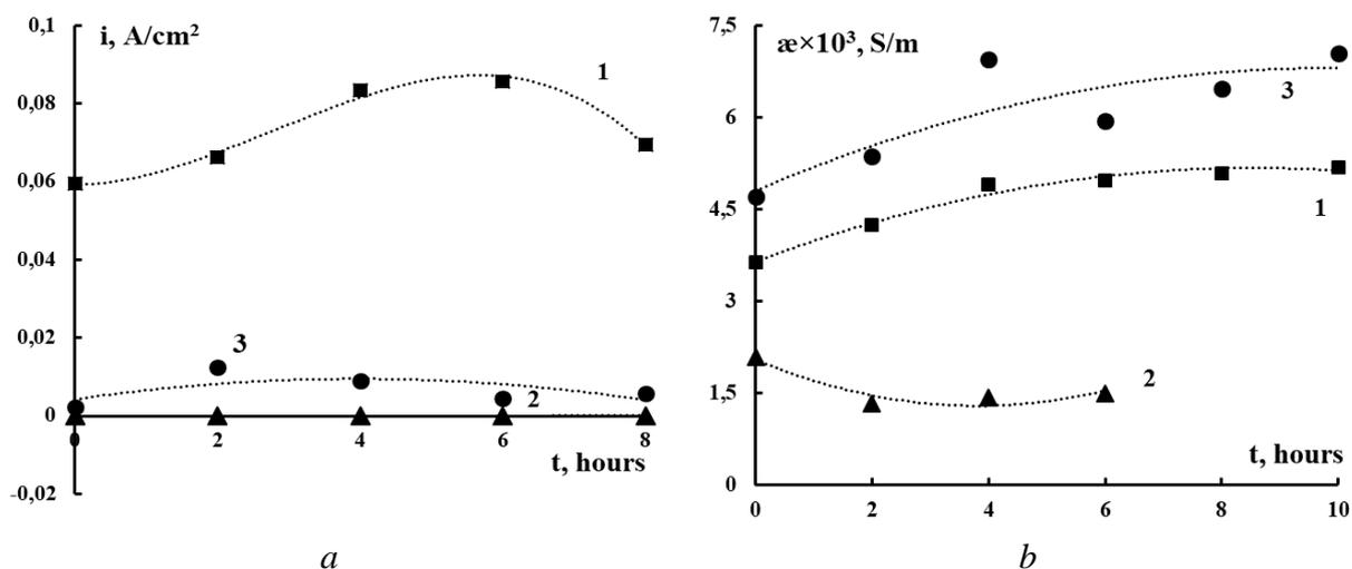
Figure 1. The time dependence of current density(a) and dependence of the electrical conductivity of the MEA on time at a potential difference of 0.5 V (b); 1.E-TEK-CI-40 (Pt); 2.Cu/C; 3.PtCu<sub>2.8</sub>/C.
