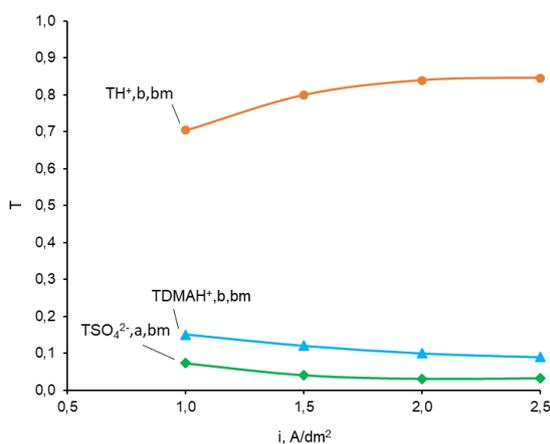
Figure 4. The dependence of the effective transport numbers of ion through the bipolar membrane depending on the electric current density in the system " dimethylamine, dimethylamine sulfate–H<sub>2</sub>SO<sub>4</sub>».
