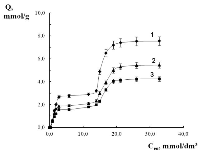
Figure 1. Adsorption Isotherms of  $\alpha$ -tocopherol on acid-activated clinoptilolite from solution:
