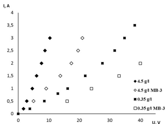
Figure 2. Current-voltage characteristics of a pair chamber, where :  $\blacklozenge$  - model solution (salt content 4.5 g/L) with experimental bipolar membranes,  $\diamond$  - model solution (salt content 4.5 g/L) with MB-3 bipolar membranes,  $\blacksquare$  – softened water (salt content 0.35 g/L) with experimental bipolar membranes,  $\square$  – softened water (salt content 0.35 g/L) with MB-3 bipolar membranes.
