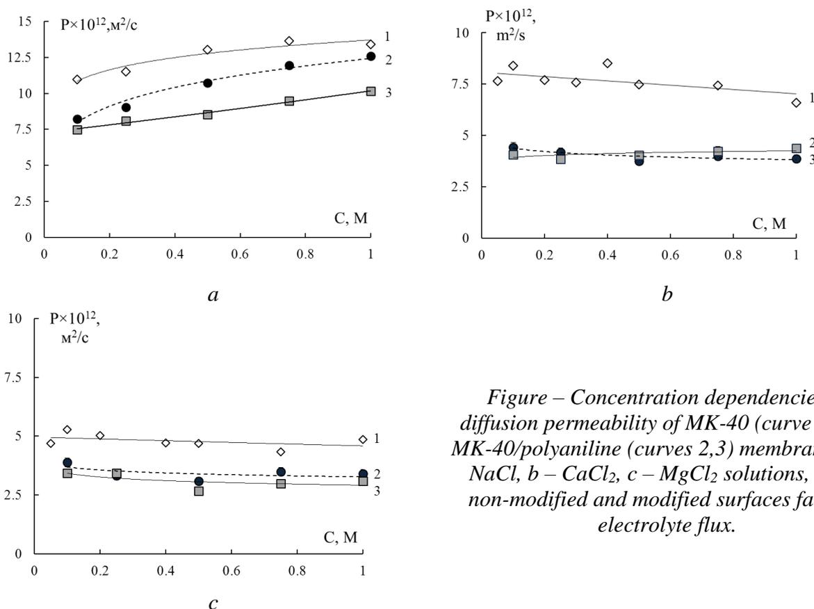
Figure – Concentration dependencies of diffusion permeability of MK-40 (curve 1) and MK-40/polyaniline (curves 2,3) membranes: a – NaCl, b – CaCl<sub>2</sub>, c – MgCl<sub>2</sub> solutions, 2, 3 – non-modified and modified surfaces face the electrolyte flux.
