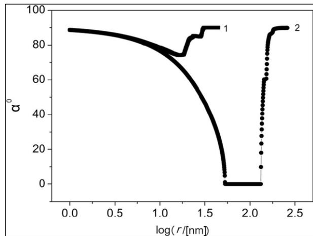
Figure 2 Wetting angle for water as a function of pore radius. Materials are the Norit carbon powder (1) and the electrode based on carbon Norit (2).
