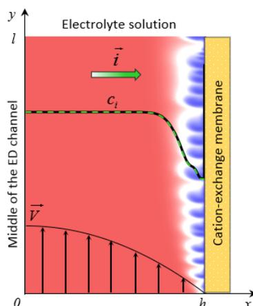
Figure 1. Scheme of the system under consideration: half of the ED cell adjacent to the CEM. Schematic concentration profiles of cations ( $c_1$ , solid line) and anions ( $c_2$ , dashed line), direction of the electric current  $\vec{i}$ , forced flow velocity  $\vec{V}$ , electroconvection vortices (blue color) are shown.
