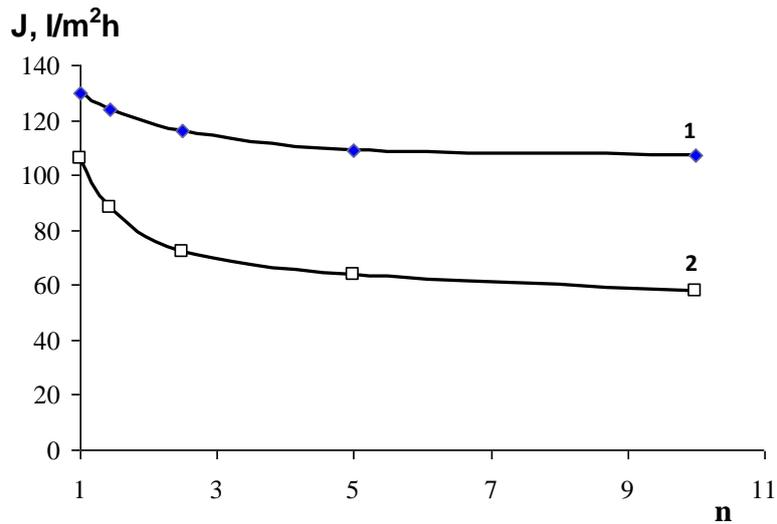
Figure. Typical dependence of transmembrane flux ( $J$ ) vs. degree of concentration ( $n$ ): 1 – ultrafiltration with mixture high basic aluminium polyoxychloride/PDMDAAC, 2 – ultrafiltration without coagulant.
