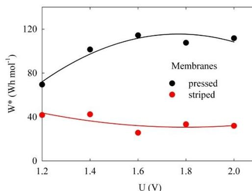
Figure 3. Dependence of specific energy costs on voltage for CDI with pressed and with striped membranes at a flow rate of 15 cm<sup>3</sup>/min.
