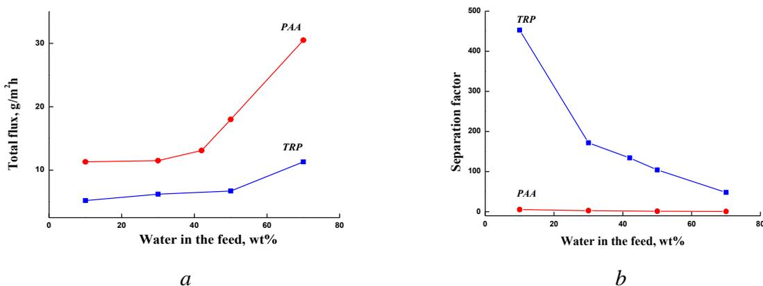
Figure 3. Dependence of (a) total flux and (b) separation factor on water content in the feed in pervaporation of water – n-butanol mixture using PAA and TRP membranes, 20°C.
