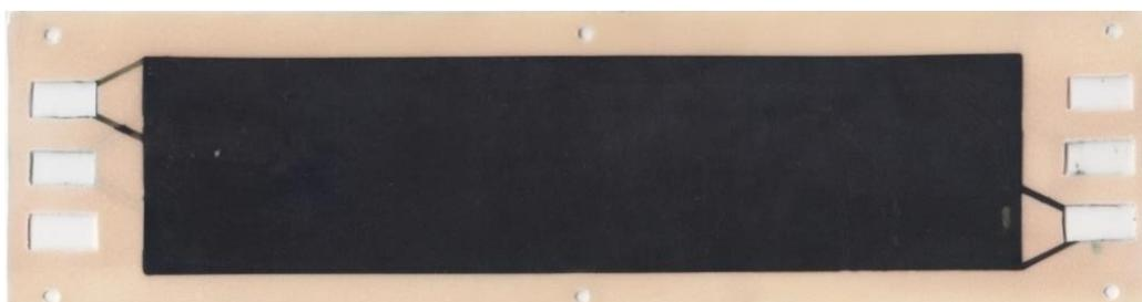
Figure 3. Image of the membrane MK-40 modified by polyaniline (active area  $5 \times 20 \text{ cm}^2$ ).
