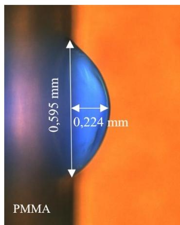
Figure 2. Pristine DOWEX™ HCR-S/S particle in a polycarbonate microcell before the experiment.
