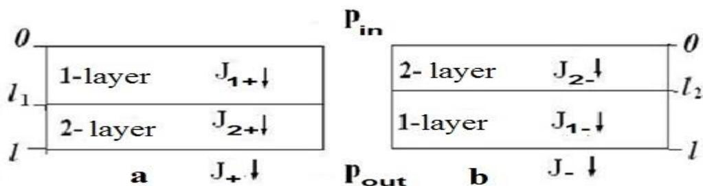
Figure 1. The scheme of gas diffusion through inhomogeneous bilayer membrane.
