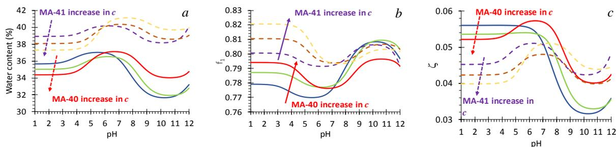
Figure 2. Water content (a), fraction of the “gel” phase (b) and the “tortuosity coefficient” in MA-40 and MA-41 membranes as functions of pH. Concentration of NaCl bathing solution is 0.1, 0.5 and 1 M.
