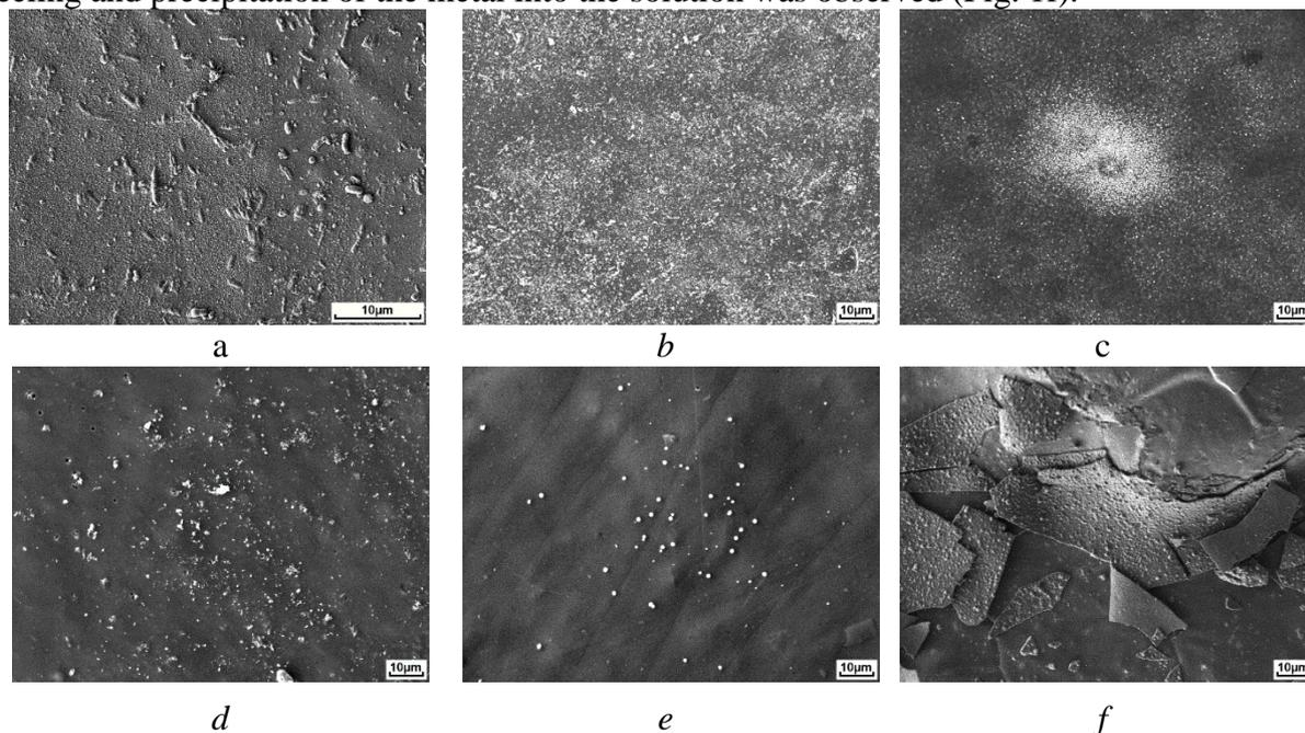
Figure 1. SEM-images of modified surface of hybrid membranes MF-4SK/Pt: a-f - samples 1-5, 7 in Table 1, respectively.
