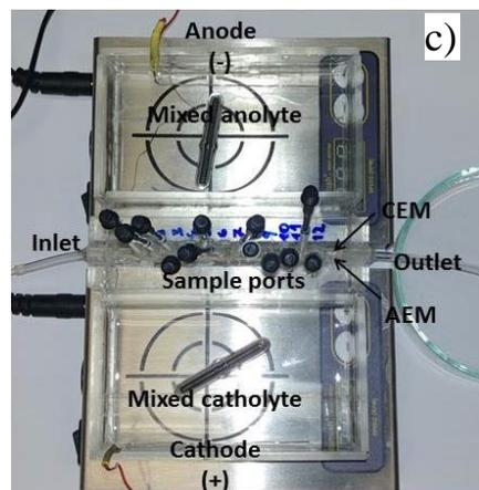
Figure 2. Various mili and microfluidic systems used in our research: a) chip for measurement of electric potential profiles in an ICP based chip, b) chip for characterization of ion-exchange systems under static conditions, c) chip for investigation of desalination under forced convection.
