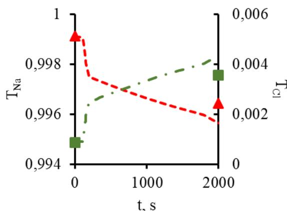
Figure 2. Time Dependence of Transport Numbers. Triangle and square dots present transport numbers of counter-ions ( $\text{Na}^+$ ) and co-ions ( $\text{Cl}^-$ ), respectively, obtained by approximate analytical solution, and lines present numerical calculations (dashed red line –  $\text{Na}^+$ , dash-dotted green line –  $\text{Cl}^-$ ).
