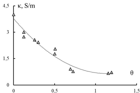
Figure 3. Dependence of the membranes conductivity on the saturation degree of the membrane with copper ions in solutions of copper sulfate.
