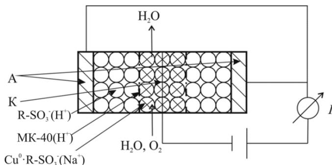
Figure 1. Sorption-membrane electrolytic cell scheme.
