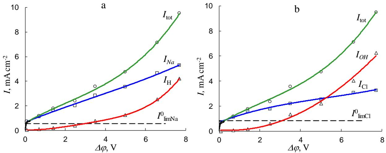
Figure 1. Current-Voltage Curves for the Diluate Compartment Formed of the Cation-Exchange Membrane MK-40 and the Anion-Exchange Membrane MA-40 in 0.002 M NaCl Solution. The total current and partial currents of  $Na^+$  and  $H^+$  ions through the MK-40 membrane (a) and partial currents of  $Cl^-$  and  $OH^-$  ions through the MA-40 membrane (b) are shown. The data are taken from [5].
