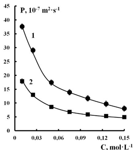
Figure 2. Dependences of the integral coefficients for the diffusion permeability of the membranes MK-40<sub>pr</sub> (1) and MA-40<sub>pr</sub> (2) on the concentration of the phenylalanine solutions.
