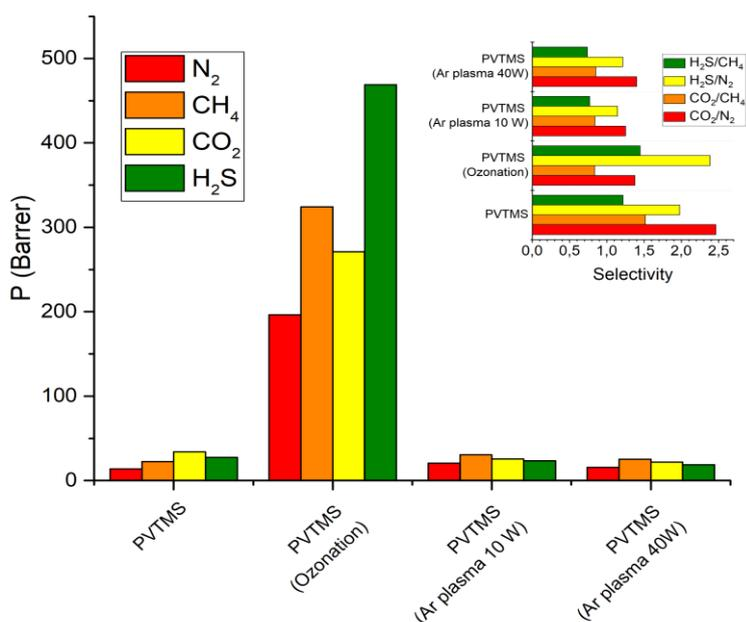
Figure 1. Permeability coefficient and ideal selectivity of the initial and modified PVTMS membranes.
