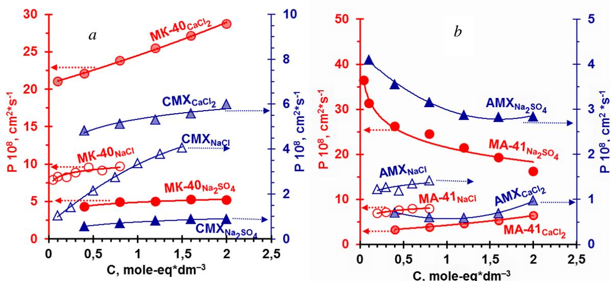
Figure 1. Concentration Dependences of Diffusion Permeability of Cation-Exchange Membranes CMX and MK-40 (a), Anion-Exchange Membranes AMX and MA-41 (b) in NaCl, CaCl<sub>2</sub> and Na<sub>2</sub>SO<sub>4</sub> Solutions.
