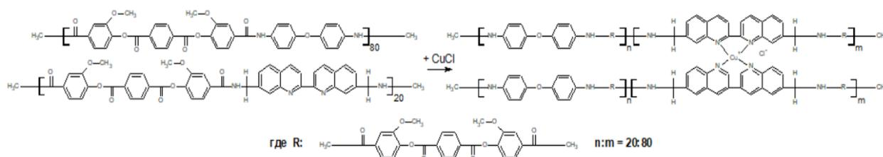
Figure 1. Scheme of PA to PA-Cu(I) transformation.
