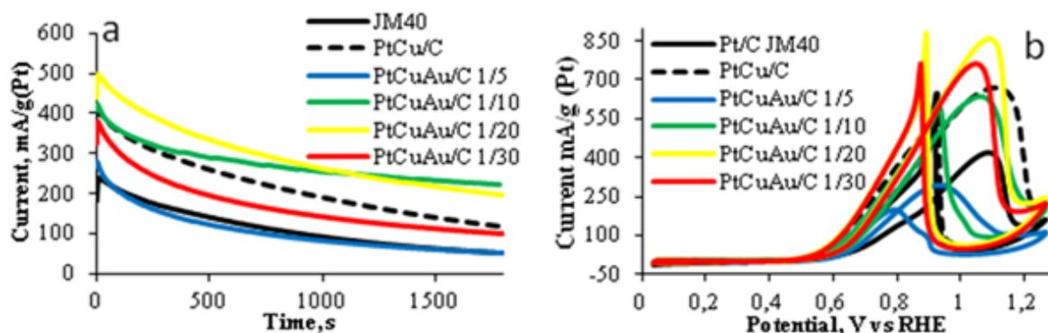
Figure 2. (a) Chronoamperograms and (b) Cyclic voltammograms to Pt/C and PtCuAu/C catalysts, electrolyte 0.1M HClO<sub>4</sub> + 0.5M CH<sub>3</sub>OH, saturated with argon, at atmospheric pressure; potential sweep rate 20 mV/s.
