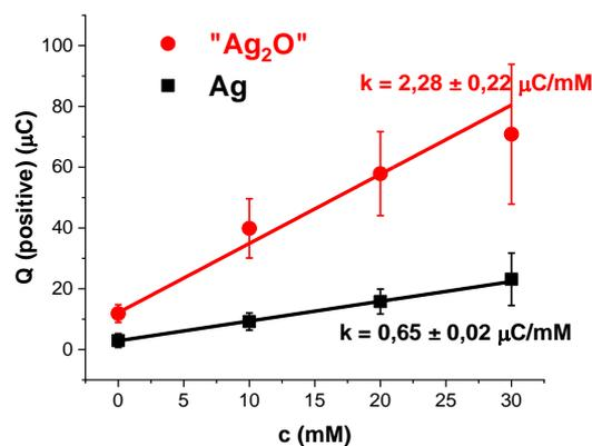
Figure 2. Linear dependence between the positive charge and acetaldehyde concentration for Ag and Ag-pretreated electrodes.
