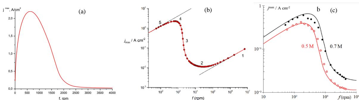
Figure 1. Dependence of the maximal current density of the bromate reduction for RDE under steady-state conditions on the electrode rotation frequency. Theoretical predictions (a) and (b).
