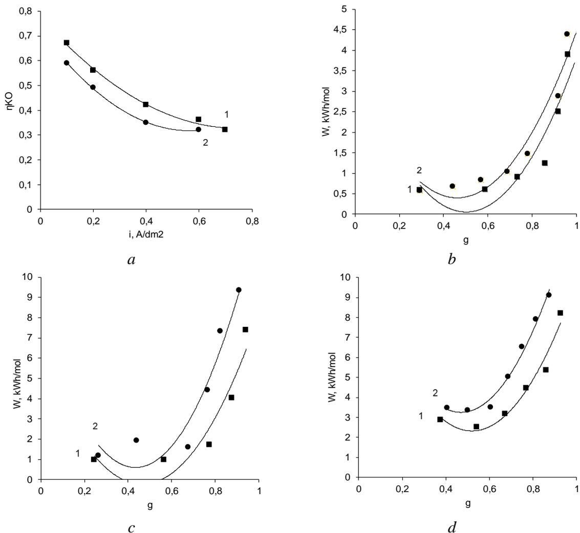
Figure 3. Current efficiency vs current density (a) and specific energy consumption vs desalting degree at 0.32 (b), 0.64 (c), 0.96 (d)  $A/dm^2$ . Desalination channel width: 1 – 0.9 mm; 2 – 1.9 mm.
