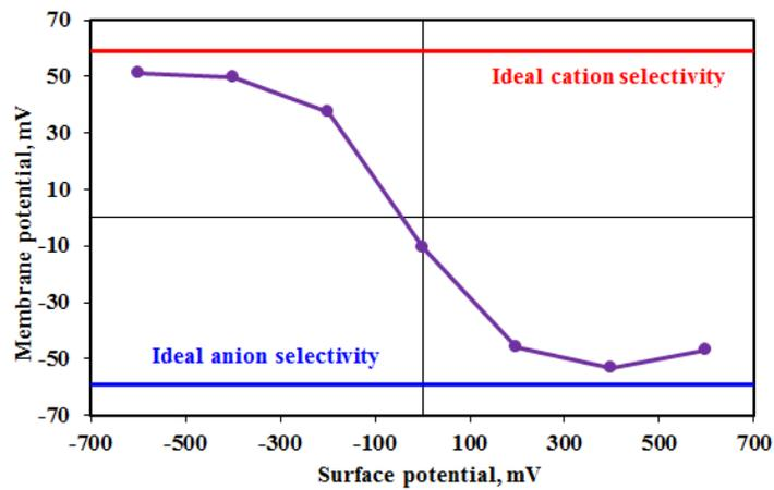
Figure 2. The dependence of membrane potential on the potential applied to the membrane surface.  $C_L=10\text{ mM}$ ,  $C_R=1\text{ mM}$ . The lines correspond to ideal cation and anion selectivity.
