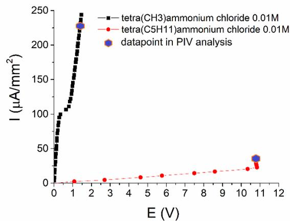
Figure 5. CVC complementary to the velocity maps for DOWEX™ HCR-S/S particle in the solution of tetramethyl and tetrapentylammonium chlorides 0,01M.
