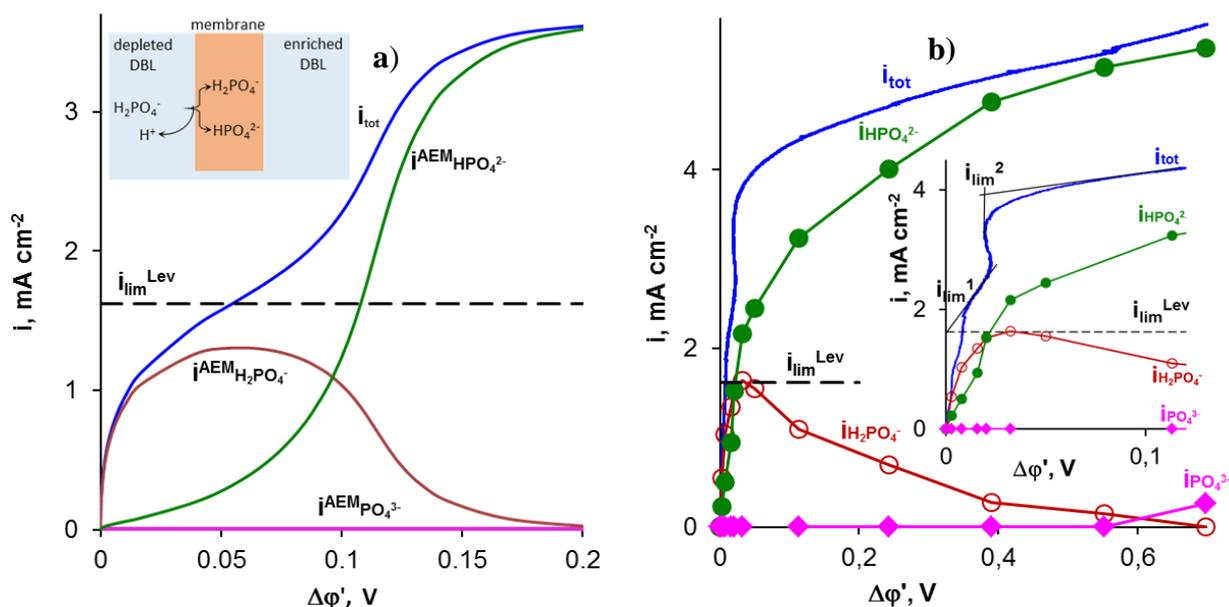
Figure 2. Total and Partial Current-Voltage Characteristics of AMX Membrane in 0.02 M  $\text{NaH}_2\text{PO}_4$  Solution: Calculation Using Model (a), Experiment (b). The dashed line is the limiting current calculated using the Leveque equation.
