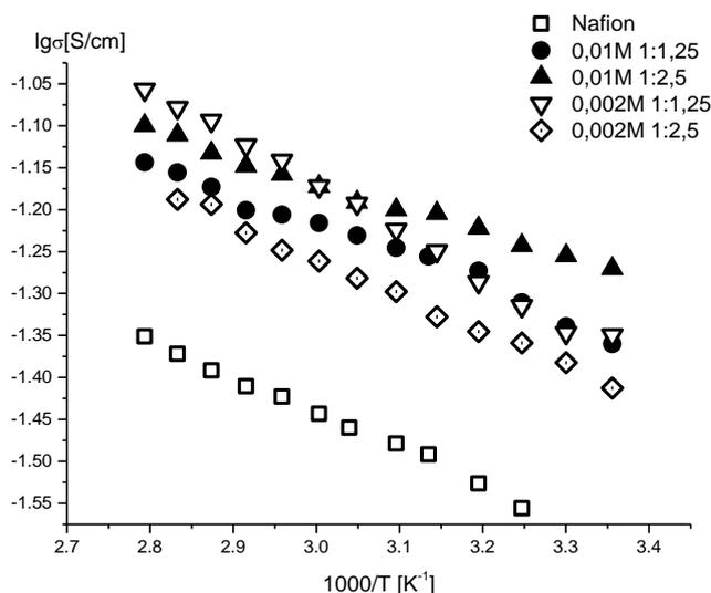
Figure. The dependence of conductivity on temperature for the obtained composite membranes. The monomer concentrations used and the monomer/oxidizer ratio are denoted in the Figure.
