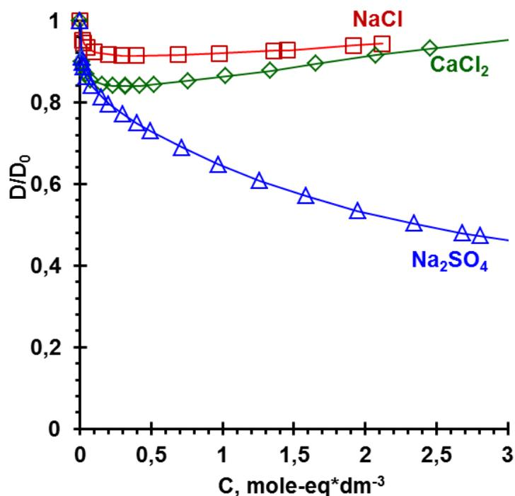
Figure 2. The Concentration Dependence of the Diffusion Coefficient of the Electrolyte  $D$  at the Temperature 25°C. Values of  $D$  normalized to the diffusion coefficient corresponding to each electrolyte at infinite dilution of the solution,  $D_0$ ). The curves are plotted from experimental data taken from [5,6].
