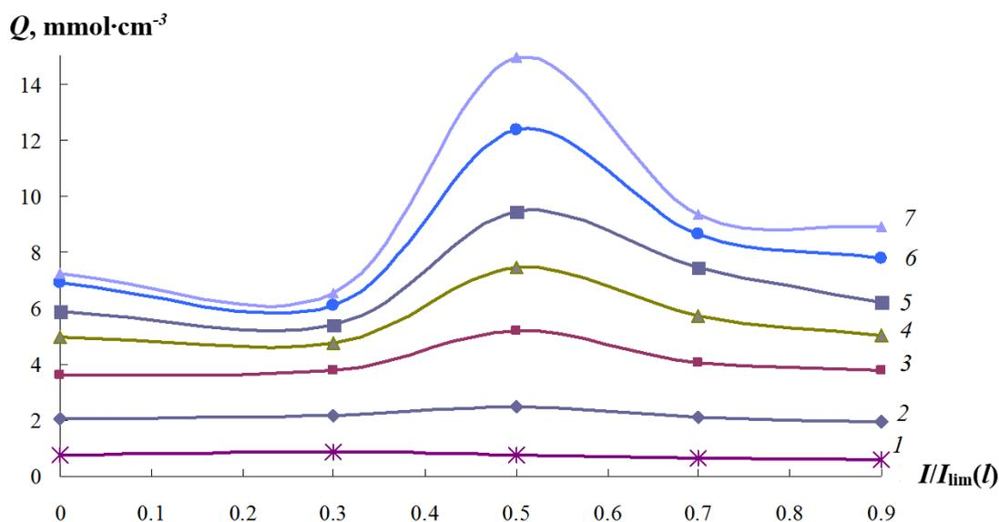
Figure 3. Reduction oxygen quantity on  $\text{Cu}^0\text{-Lewatit K2620}(\text{Na}^+)$  nanocomposite at the time  $t$ , h: 1 – 5; 2 – 15; 3 – 30; 4 – 45; 5 – 60, 6 – 80; 7- 100. Experiment conditions:  $l=6 \cdot 10^{-2}$  m  $u=0.23$  cm/sec,  $c_0=8.1 \pm 0.2$  mg/l,  $I_{\text{lim}}(l)=12.3$  mA.
