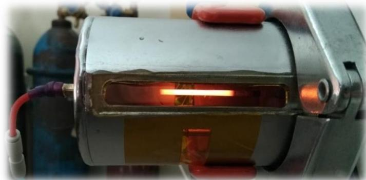
Figure 1. Direct AC/DC heating of hollow fiber membranes.
