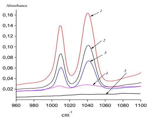
Figure 3. ATR-FTIR-spectra of UHMWPE-sPS membranes in the  $\text{Na}^+$  form. The PS content in the composites are 36 (1), 27 (2), 15 (3), and 7 (4) wt. %. 5 – the initial UHMWPE film.
