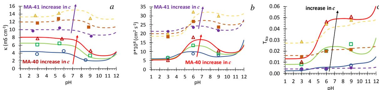
Figure 1. pH dependencies of electric conductivity (a), local coefficient of diffusion permeability (b) of MA-40 and MA-41 membranes; transport numbers (c) of Na<sup>+</sup> ions in MA-40 (solid lines) and MA-41 (dashed lines) membranes. Concentration of NaCl bathing solution is 0.1, 0.5 and 1 M.
