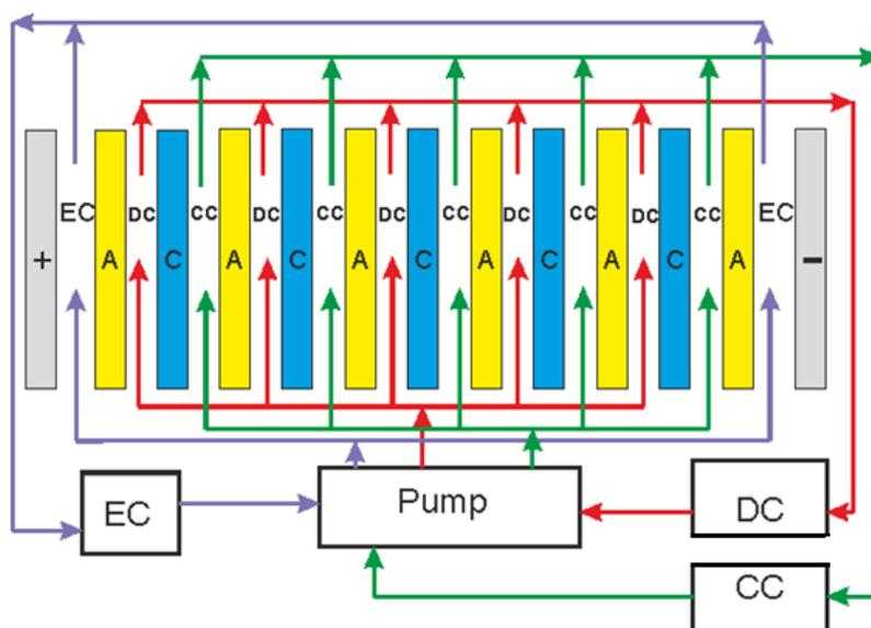
*A – anion-exchange membrane; C – cation-exchange membrane;*
