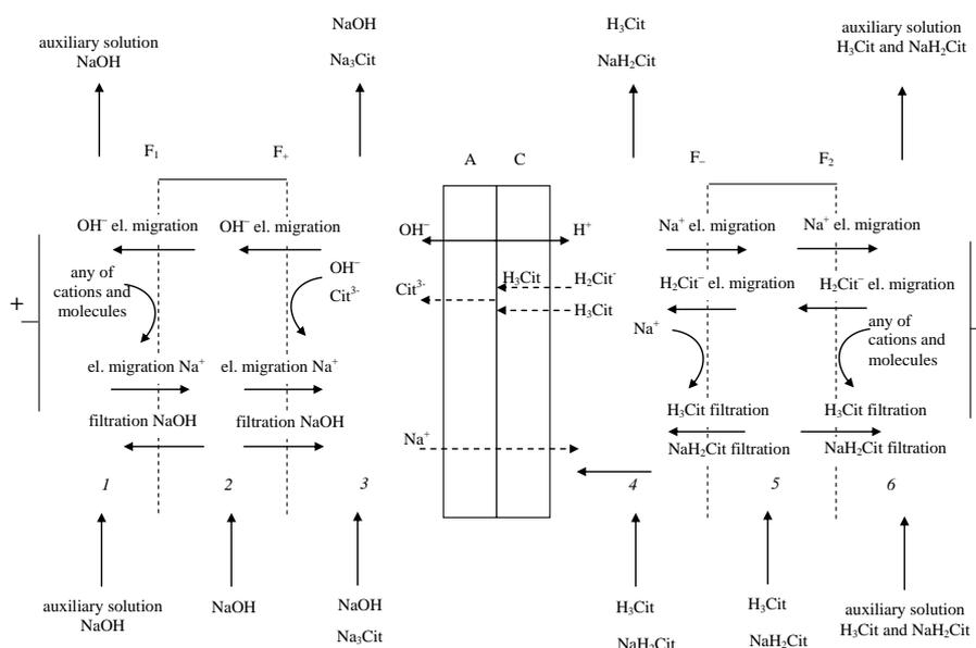
Figure 1. Scheme of ions and molecules transfer processes through the investigated bipolar membrane in the system "alkali solution – solution of citric acid and sodium citrate».
