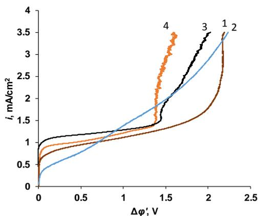
Figure 2. General current-voltage characteristics of ion-exchange membranes in 0.02 M NaCl solution. 1 - Ralex AMH, 2 - Ralex/MF-4SK, 3 - Ralex/PANi, 4 - Ralex/MF-4SK/PANi.
