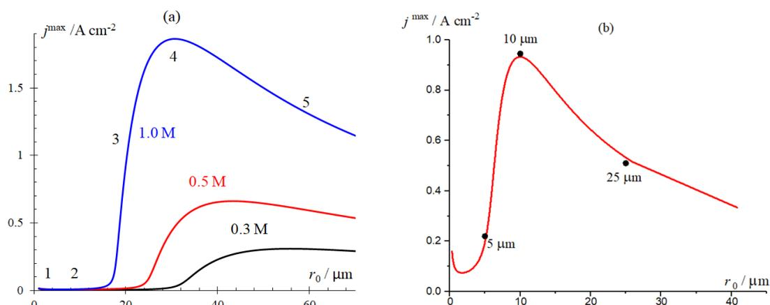
Figure 2. Dependence of the maximal current density,  $j^{\max}$ , of a microelectrode on: (a), (b) its radius or (c) on its inverse radius,  $r_0^{-1}$ . Graphs (a) theoretical predictions for various bulk-solution concentration of  $\text{BrO}_3^-$ ; (b), (c) experimental data for  $0.2\text{M NaBrO}_3 + 4\text{M H}_2\text{SO}_4$  (points) vs. theoretical line.
