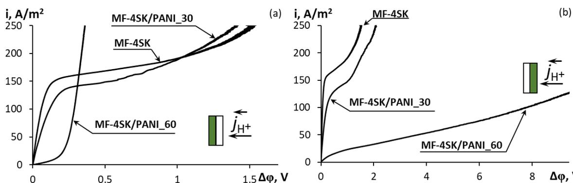
Figure 2. I-V curves of pristine MF-4SK membrane and membranes synthesized during 30 (MF-4SK/PANI\_30) and 60 (MF-4SK/PANI\_60) min: unmodified (a) and modified (b) surface layer was placed towards the desalination compartment.
