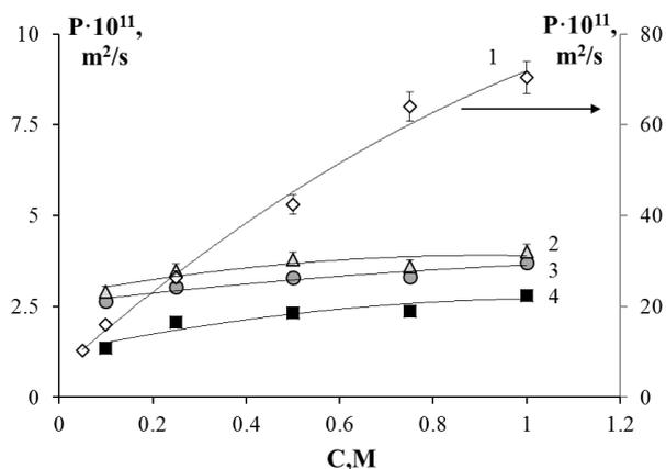
Figure 1. Concentration dependencies of the membrane diffusion permeability in NaCl solutions. 1 – MF-4SK, 2, 3 – non-modified and modified surfaces of MF-4SK/PANI membrane faces the electrolyte flux, 4 – bulk-modified sample.
