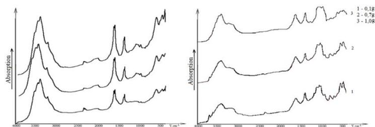
Figure 4. IR-spectra of the studied samples obtained by sorption of iron ions (a) and cobalt (b) at different sorbent norm.
