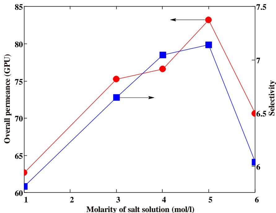
Figure 1. The overall permeance of ethylene and ethylene/ethane selectivity as a function of  $\text{AgNO}_3$  concentration. The liquid velocity was 0.2 m/s; GPU denotes gas permeance unit,  $1 \text{ GPU} = 3.35 \cdot 10^{-10} \text{ mol}/(\text{m}^2 \cdot \text{s} \cdot \text{Pa})$ .
