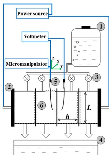
Figure 1. Schematic Representation of the Scanning Electrochemical Microscope.
