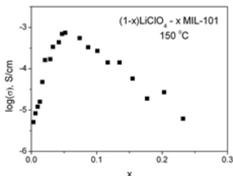
Figure 1. Concentration dependence of conductivity of the  $(1-x)\text{LiClO}_4 - x\text{CrMIL-101}$  composites.
