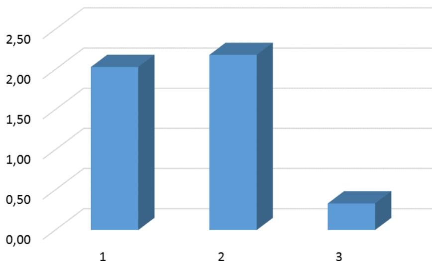
*Figure 2. The content of vanadium pentoxide  $V_2O_5$  in solutions before and after electro dialysis processing: 1 - the content of  $V_2O_5$  in the model solution is 2.03 g/l, 2 -  $V_2O_5$  content in the concentrate 2.18 g/l, 3 - the content of  $V_2O_5$  in the desalting solution 0.33 g/l.*
