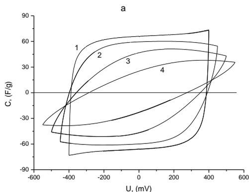
Figure 4. Capacitance of static cell with pure water as a function of voltage at different scan rate: 1 - 0.1 mV / s; 2 - 0.5 mV / s; 3 - 2 mV / s; 4-5 mV / s.. Pure water, AC Norit , mosaic film membrane.
