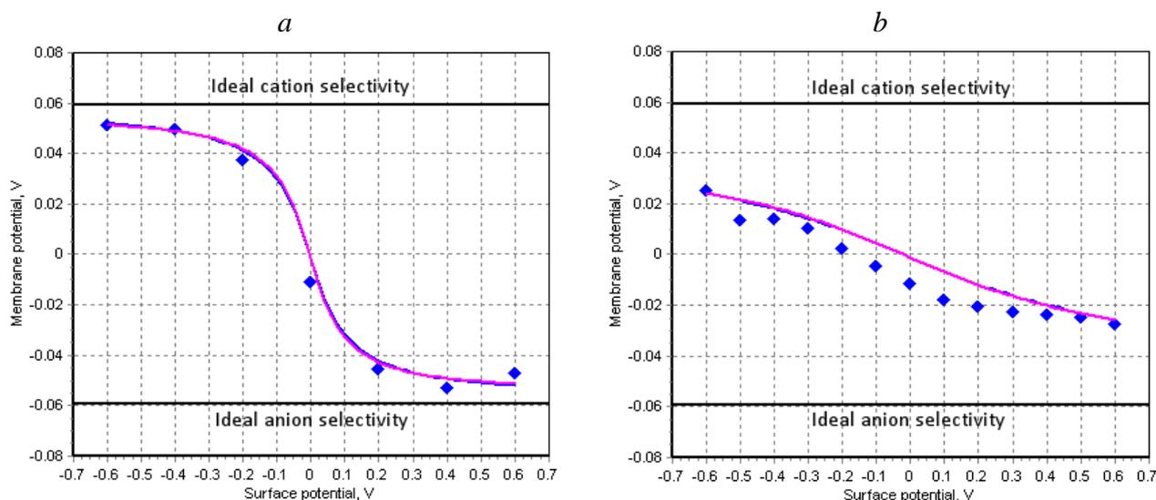
Figure 1. The dependence of membrane potential on the surface potential for KCl aqueous electrolyte with  $C_L=10$  mM,  $C_R=1$  mM (a) and  $C_L=100$  mM,  $C_R=10$  mM (b). Experiment (dots) and theoretical models (blue curves – 2D, magenta curves – 1D). The fitted value of pore radius is 12.9 nm (a) and 11.0 nm (b), pore lengths is 400  $\mu$ m.
