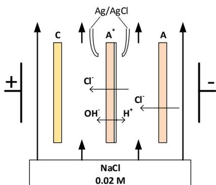
Figure 1. The scheme of the experimental cell and ions fluxes through the studied membrane. C – cation-exchange membrane MF-4SC; A – anion-exchange membrane MA-41; A\* – membrane under study.
