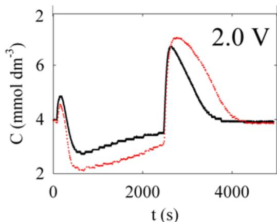
Figure 2. Dependence of KCl concentration on deionization time and concentration for a flow of 15 cm<sup>3</sup> / min and voltage 2 V for pressed (black) and striped (red) membranes.
