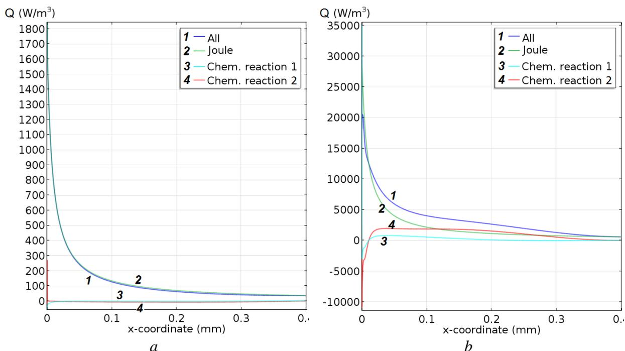
Figure 3. Heat sources for  $\text{NaH}_2\text{PO}_4$  solution with concentration  $1 \text{ mol/m}^3$  (a) and  $20 \text{ mol/m}^3$  (b) at a given potential drop in the diffusion layer  $d_\phi = -0.2V$ .
