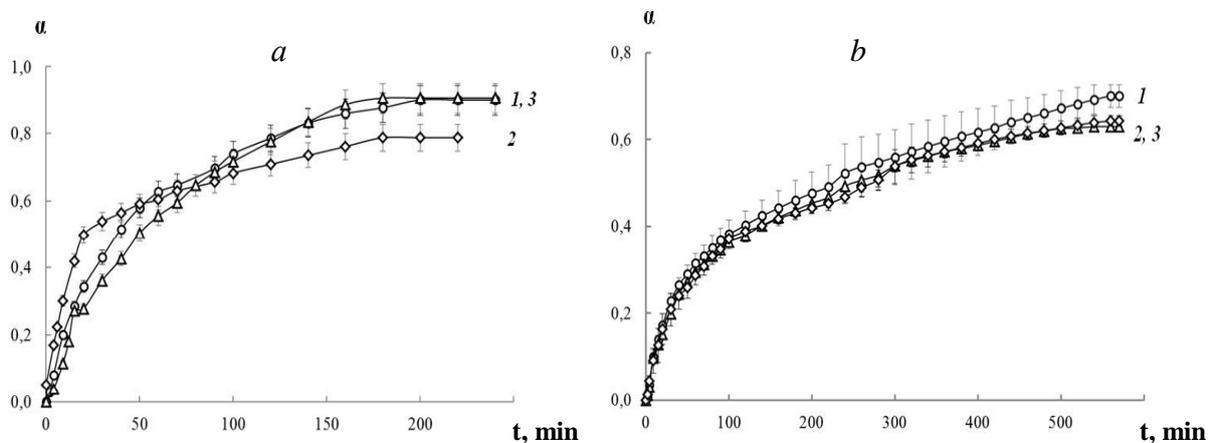
Figure 1. Kinetic curves for the degree of absorption of oxygen  $\alpha$  from water as a function of time  $t$  by nanocomposites: 1 - Cu·KY-23( $H^+$ ), 2 - Cu·Lewatit SP-112  $H(H^+)$ , 3 - Cu·Lewatit K 2620( $H^+$ ) with various cycles of deposition of copper; a)  $N=1$  b)  $N=5$ .
