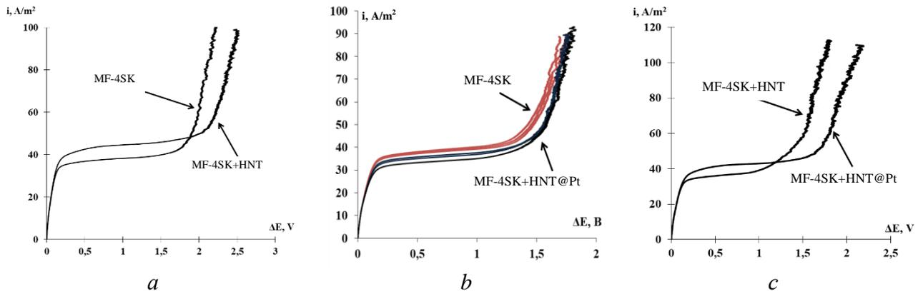
Figure 2. Current voltage curves of bi-layer membranes MF-4SK/MF-4SK+ HNT (a), MF-4SK/MF-4SK+ HNT@Pt (b) and MF-4SK+HNT/MF-4SK+HNT@Pt (c). Arrows point out the side of membrane where the limiting state occurred.
