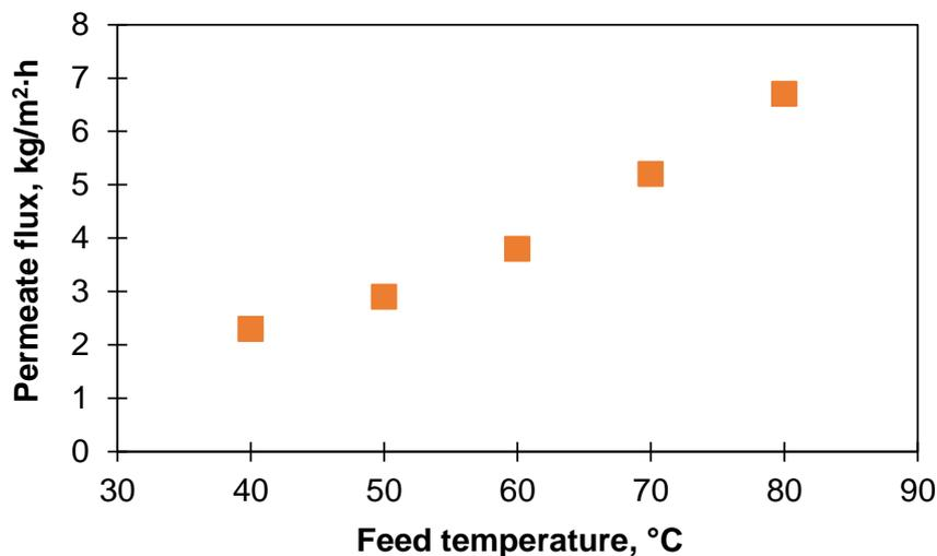
Figure 2. Dependences of permeate flux on feed temperature for 50 g/l NaCl solution,  $T_c = 20^\circ\text{C}$ ,  $l_{\text{air gap}} = 2.5 \text{ mm}$ .
