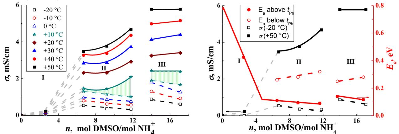
Figure 2. Ionic conductivity and activation energy of conductivity above and below the phase transition temperature  $t_{ph}$ , depending on the content of DMSO in ammonium substituted membranes.
