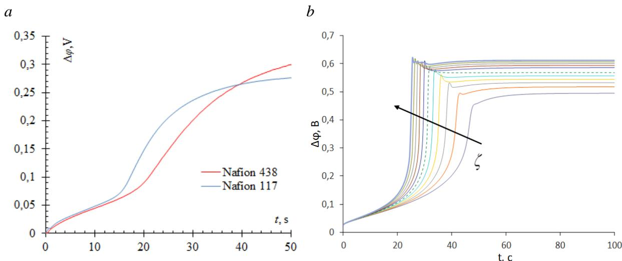
Figure 1. Experimental Chronopotentiograms for Nafion 117 and Nafion 438 Membranes (a) and Calculated Chronopotentiograms Using the Developed 2D Mathematical Model (b) ( $\zeta$ -potential values were changed in the range from  $-0.5$  to  $0.5$  V, the direction of increase  $\zeta$  is indicated by an arrow, the dashed line indicates the chronopotentiogram for  $\zeta = 0$  V) at  $j = 1.25j_{lim}$ .
