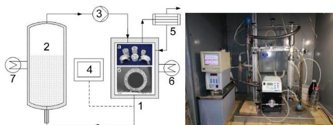
Figure 1. Lab-scale set-up for CO<sub>2</sub> desorption from MEA solution: 1- desorption unit (a - small stripping column with Rashig rings ( $\varnothing$  6 mm); b - membrane gas-liquid contactor with hollow fibers); 2 - solvent tank with CO<sub>2</sub>-rich MEA solution; 3- solvent gear pump; 4 - temperature control unit; 5 - condenser; 6 - heater (thermostate); 7- cooler (tap water).
