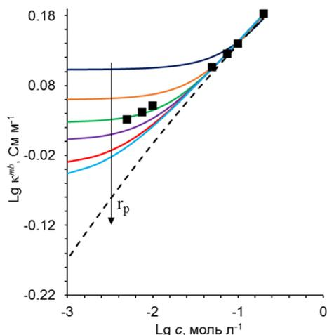
Figure 1. Experimental (dots) and Calculated (lines) Concentration Dependences of the Membrane Conductivity in NaCl Solutions. Calculations are made for pores with a flat geometry. The dashed line is the prediction of the base microheterogeneous model [1]; solid lines - prediction of the modified microheterogeneous model. The arrow shows the direction of increase  $r_p = 1, 3, 6, 10, 20, 30$  nm.
