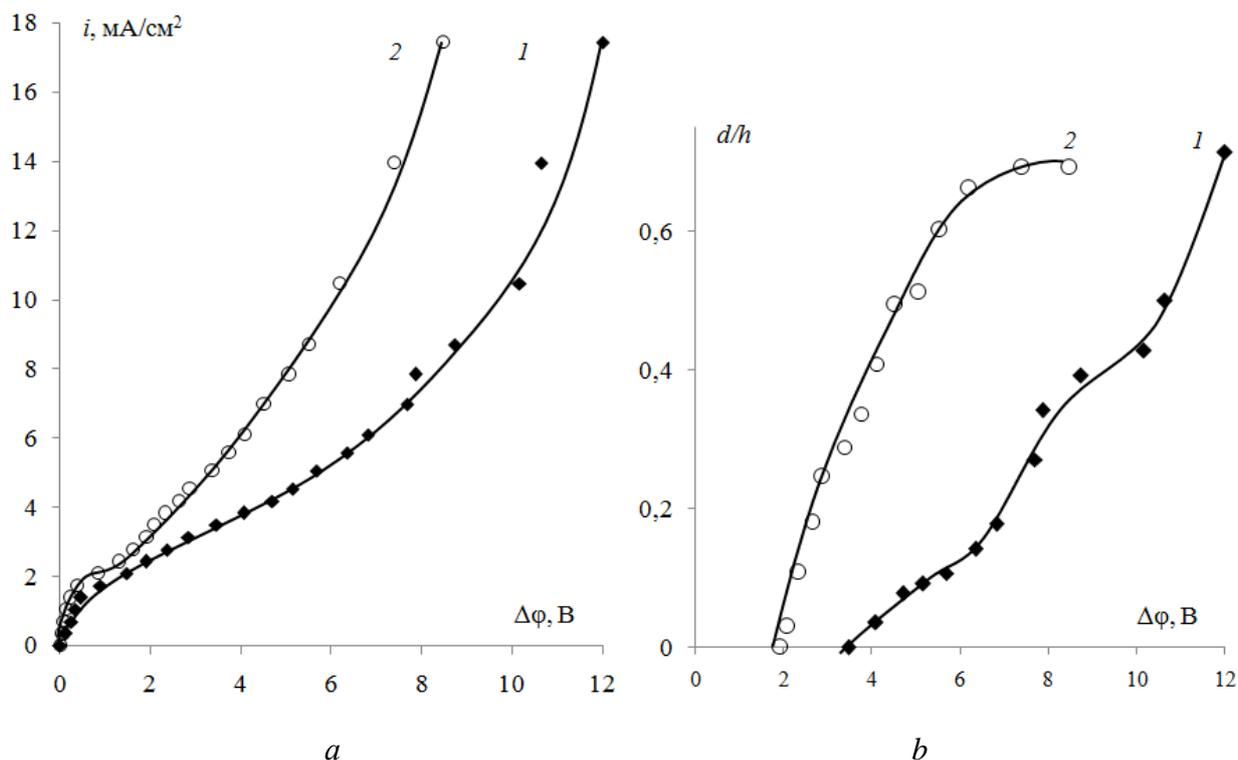
Figure 1. Current-voltage curves (a) and thickness of the convective instability region normalized to the intermembrane distance  $h$  (b) in solution at the boundary with cation-exchange membranes with the sulfonation-exchanger fraction of 45 % (1) and 70% (2).
