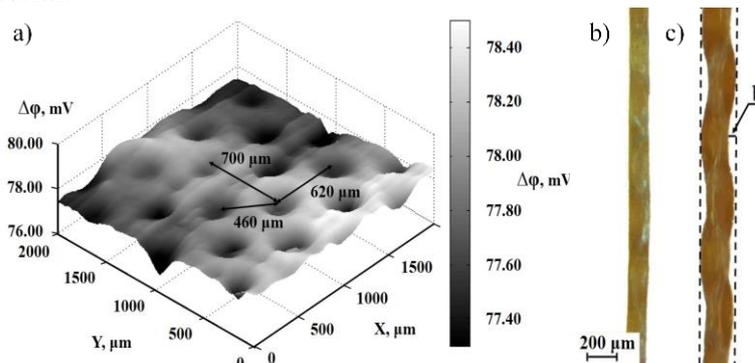
Figure 2. Potential Drop Distribution Near the Surface of the CMX Membrane (a), Optical Cross Section Images of the Dry (b) and Swollen (c) CMX Membrane.
