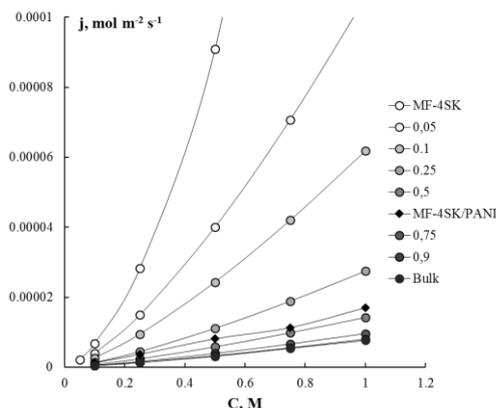
Figure 3 – Concentration dependencies of the diffusion flux in NaCl solutions. 0.05, 0.1, 0.25, 0.5, 0.75, 0.9 – calculation results (curve number defines the  $q_2$  value), MF-4SK, MF-4SK/PANI and Bulk – experimental data for initial, surface- and bulk-modified samples correspondingly.
