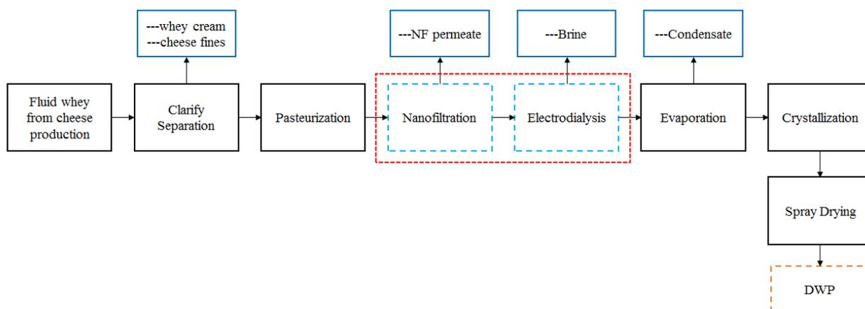
Figure 2. NF and ED flow diagram.
